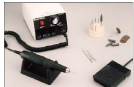
Figure 1: Drill out the hole using a Micro-Drill System and ball mill.
