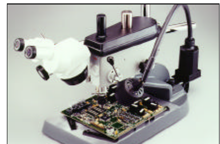
Figure 1: Precision Drill System with base plate to pin PC board in position while cutting circuits.
