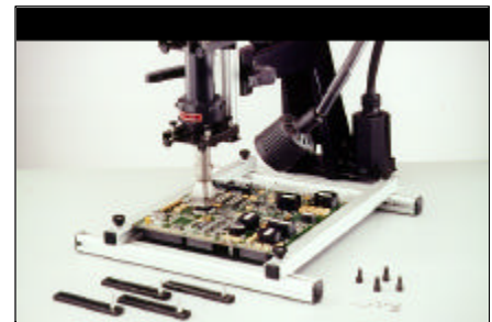
Figure 2: Rework stand holds hot air rework tool steady and positioning table keeps PC board level.
